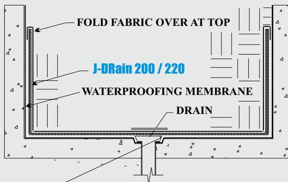
NOTE: When using J-DRain 200 / 220 cut and remove drainage core and cover with an aluminum plate as shown.
